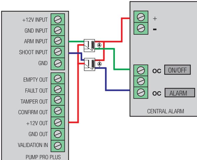
Compared to B diagram, this alarm central has only open collector outputs.
