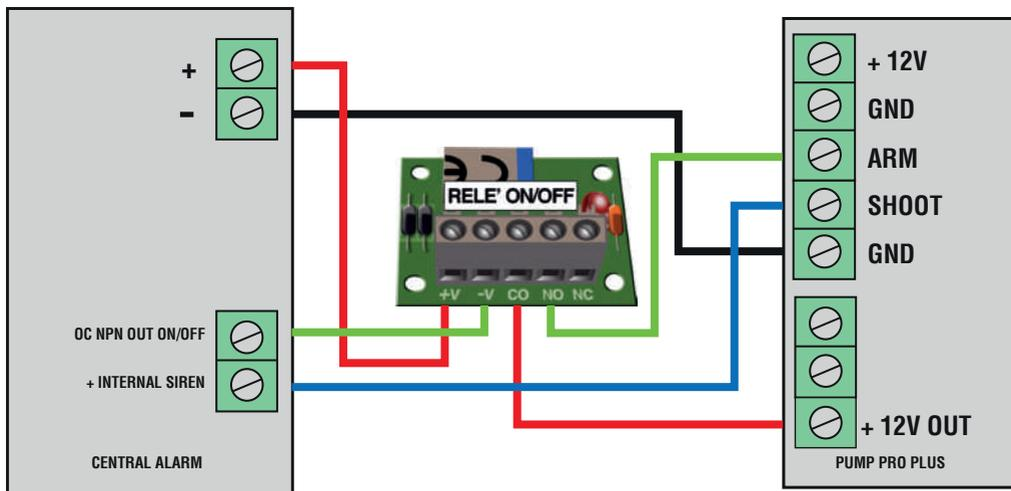
In the diagram above the control panel, as example, provides to UR Fog power supply between 11 and 14V DC 250 mA max. The ON/OFF output of this alarm is an Open Collector NPN opened when the system is off and it is stably closed to negative as long as the system turned on. The alarm output of the alarm is normally open and becomes positive during the alarm time.
