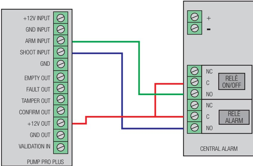
ON/OFF output of this alarm central is an open relay when the system is off and it is stably closed to positive as long as the system is turn on.
