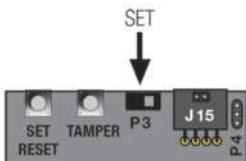
To set the shooting time, after opening the bag compartment door, at the top of the PCB, facing the board you must move the jumper in left position P3 (closer to the buttons S1/S2). Then, holding down the button S1 "SET", 6 leds on the front will flash and each flash is equivalent to 10 seconds. If you press the button again, the shooting time is not added to the one previously set, but will restart from zero.
