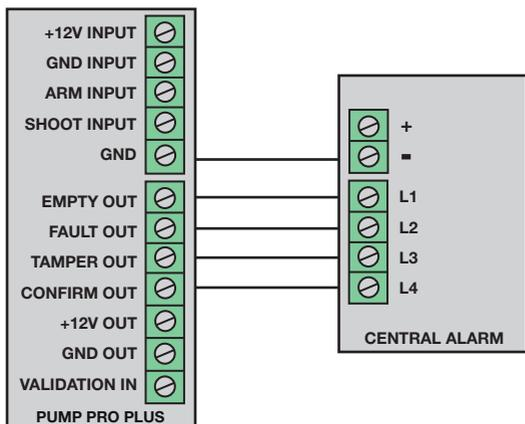
The outputs shown in the diagram are not always necessary, but only in cases where the voltage of pull-up resistance is lower than that of power supply.
