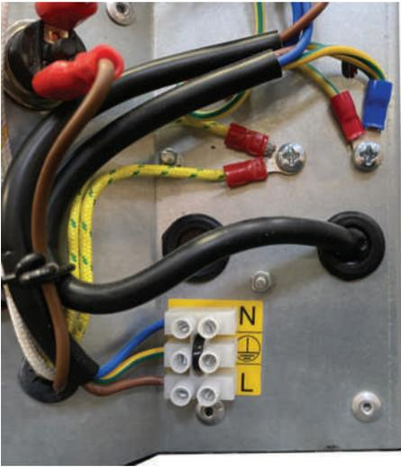
While connecting the machine to the mains power, it is recommended to never disconnect existing ground cable. The fact of disconnecting or modifying existing cables voids the warranty and can cause troubles or accidents related to the temperature control.
